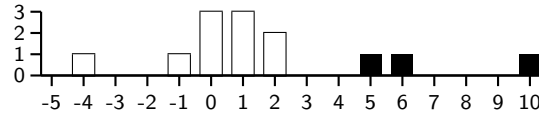
Figure 3: Frequency of confidence1 generated from Figure 2. Assumes that numeric ranges have been divided into 3 bands . Outstandingly high confidence1 values shown are in black. Y-axis is the number of ranges that have a particular confidence1 value.
