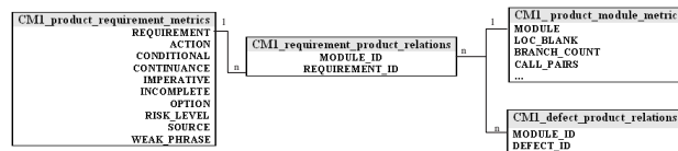
Figure 3.1. An entity-relationship diagram relates project requirements to modules and modules to faults
